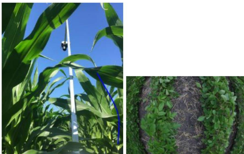
Figure 10. LAI camera suspended over corn canopy (left) and fish eye photo of a soybean crop (right)
